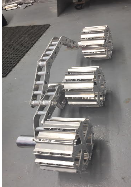
Figure 10: Manufactured Rocker and Bogie Assembly
