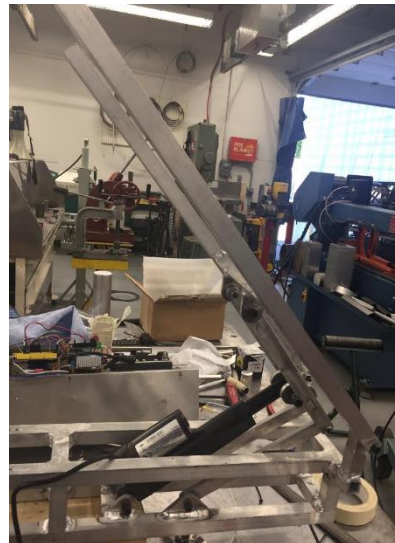
Figure 16: Manufactured Dumping Mechanism
