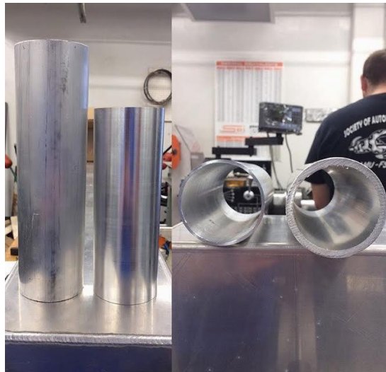
Figure 5: Before/After Machined Tubing
